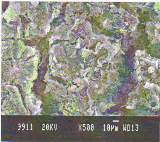
Figure 5. Microstructure of Al 7075/2% Zircon reinforced composite in sea water at 100°C and 30 minutes exposure time
